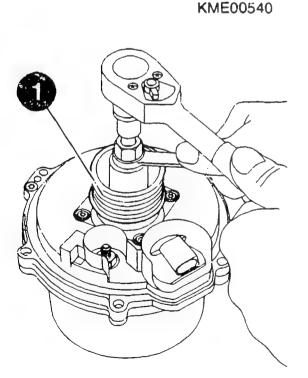
ASSEMBLING ALTERNATOR Assembling pulley (overrunning-clutch pulley) Screw overrunning-clutch pulley (1) onto rotor shaft and tighten by way of dismantling tool whilst supporting windingless rotor. Use torque wrench. 75...85 Nm Tightening torque: comm. avail. Torque wrench: 0 986 319 396 Dismantling tool: Multi-point socket M10 comm. avail. Long version:
